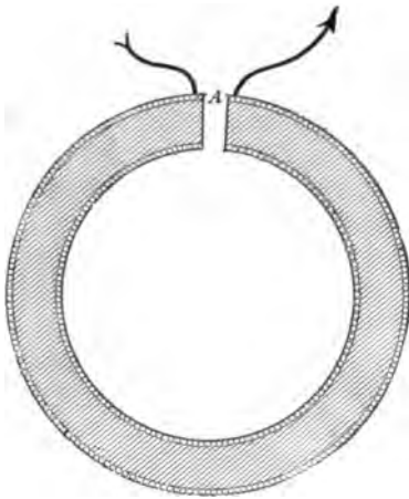
FIG. 45.—IRON RING PROVIDED WITH AIR-GAP, AND WOUND WITH WIRE.
